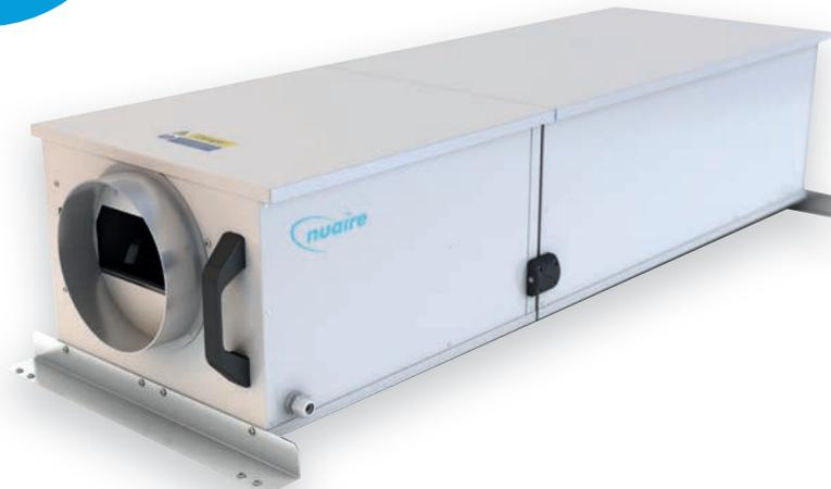
Nuaire's NOXMASTER uses Positive Input Ventilation (PIV) and houses a carbon filter cell which filters outdoor pollutants such as NO<sub>2</sub>. The unit also incorporates a PM10 pre and post filter to capture Particulate Matter caused by vehicle emissions and other industrial sources.
