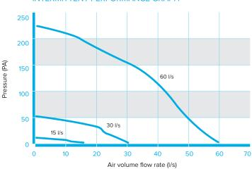
Graph shown above includes 300mm duct and low resistance external wall grille.
