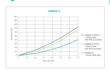
Optional pre-filters can be specified to further filter Particulate Matter and help protect the carbon filter within the IAQBOX. Choose from PM10 or PM2.5
