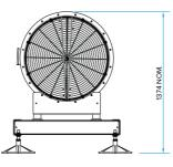
**AXH80DG-4LR ASSEMBLY WITH INLET SILENCER**
