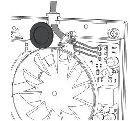
7 Cable Installation For Recessed Cable Entry
