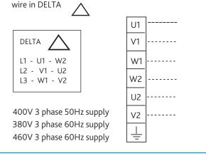
14 Wiring - Two Speed - TAP/PAM Wound Motor - D.O.L Starting (Both speeds) - Three Phase
