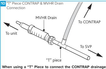
and the MVHR drain pipework the MVHR drain must always be fitted before the "T" Piece to prevent condensate from feeding back into the MVHR system.
