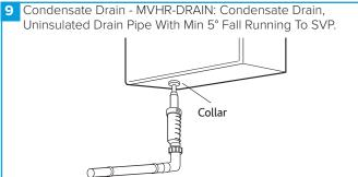
When using a "T" Piece to connect the CONTRAP drainage and the MVHR drain pipework the MVHR drain must always be fitted before the "T" Piece.
