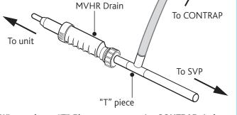
When using a "T" Piece to connect the CONTRAP drainage and the MVHR drain pipework the MVHR drain must always be fitted before the "T" Piece to prevent condensate from feeding back into the MVHR system.
