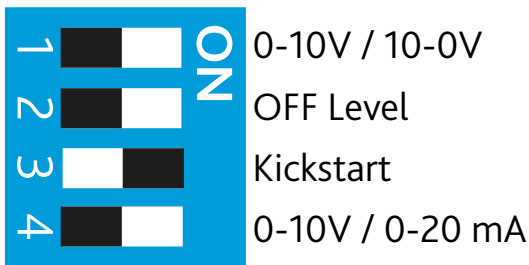
Figure 5. DIP Switch Setting
