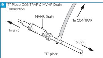
When using a "T" Piece to connect the CONTRAP drainage and the MVHR drain pipework the MVHR drain must always be fitted before the "T" Piece to prevent condensate from feeding back into the MVHR system.
