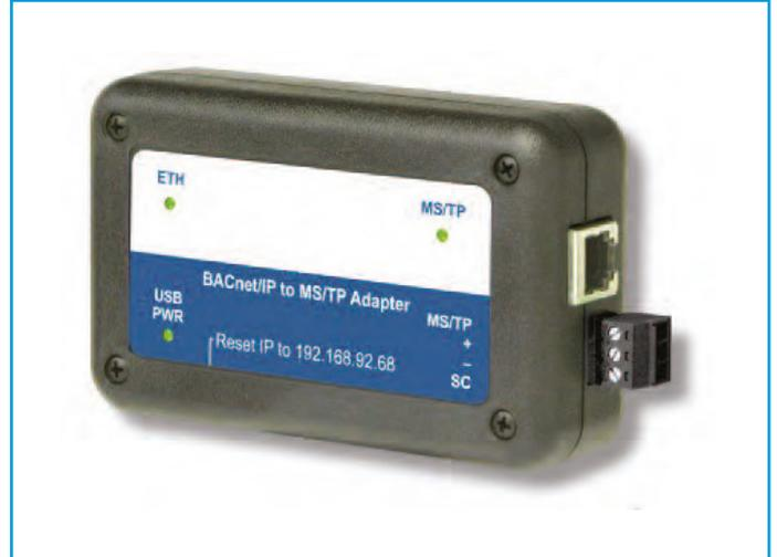
The BACnet router has a USB 2.0, Type B receptacle which is only used to obtain power from a computer or USB adapter. A mains adapter and cable is supplied. The router connects to the FC bus via screwed terminals.
