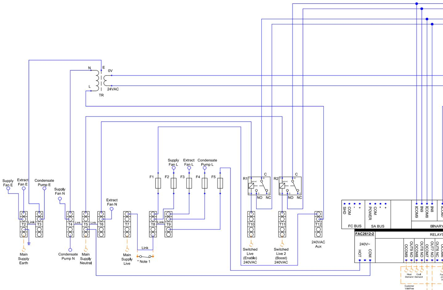
\* Note1 Emergency shutdown circuit. Break to remove power. Remove link T7-T8 to use.
