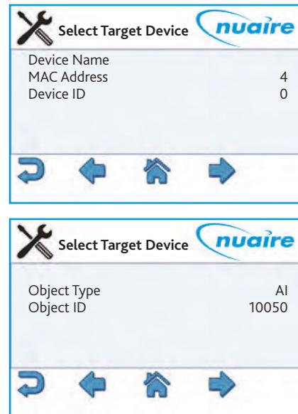
\* This is the setting of the DIP switch on the front of the FAC controller. This can also be discovered by browsing to the network screen while ID is selected in the View Config settings screen.
