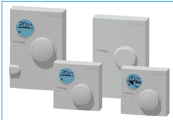
Room modules are automatically detected and require no set-up. The majority of RM modules monitor room temperature; however, options are available to also monitor zone humidity, carbon dioxide (CO<sub>2</sub>), local temperature setpoint adjustments, PIR, and other variables. This data is transmitted to a controller on the Sensor Actuator (SA) Bus.
