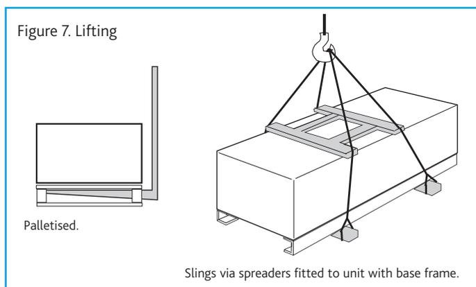
**XBOXER XBC unit sections will be delivered to site in one section.**
