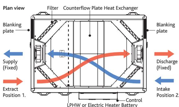
Figure 6. Bottom access only unit (Example code: XBC15-H-LCO-BA).
