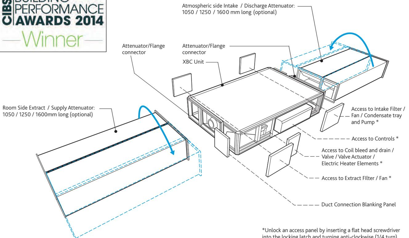
\*Unlock an access panel by inserting a flat head screwdriver into the locking latch and turning anti-clockwise (1/4 turn).
