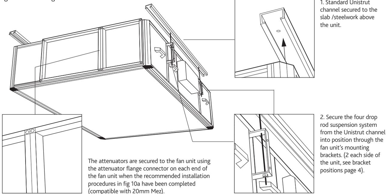
Figure 14. Installing the unit attenuators.
