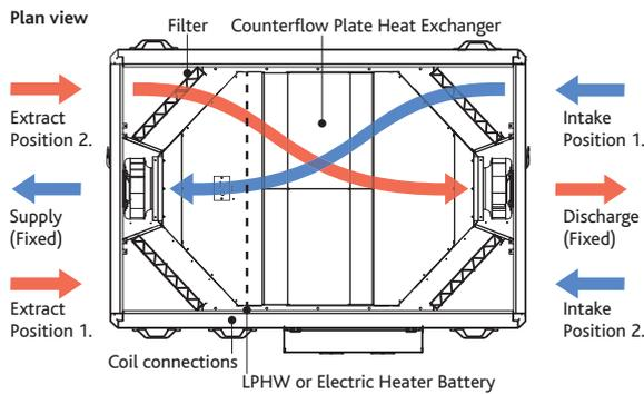
Note: The unit is shipped with four G4 filters in place, two of which are included as spares. For F7 filters contact Nuair.
