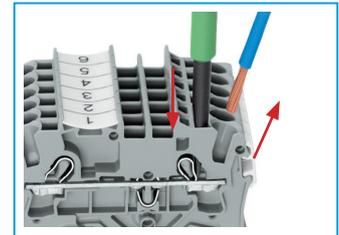
**JUMPERS** - Terminal blocks can be connected together to increase the number of terminals at the same potential using push-in jumpers. In these cases the terminals are treated as one conductor.
