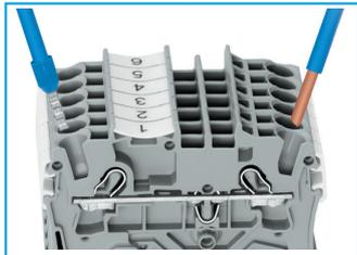
**TERMINATION OF FINE-STRANDED CONDUCTORS** - Open the clamp by inserting an operating tool (as shown below) until it clicks into position. Then insert the conductor and remove the operating tool to complete the connection.
