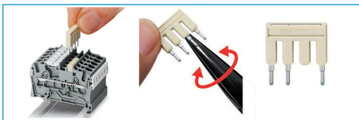
**JUMPER REMOVED** - Insert the operating tool blade between the jumper and the partition wall of the dual jumper slots, then lift up the jumper.
