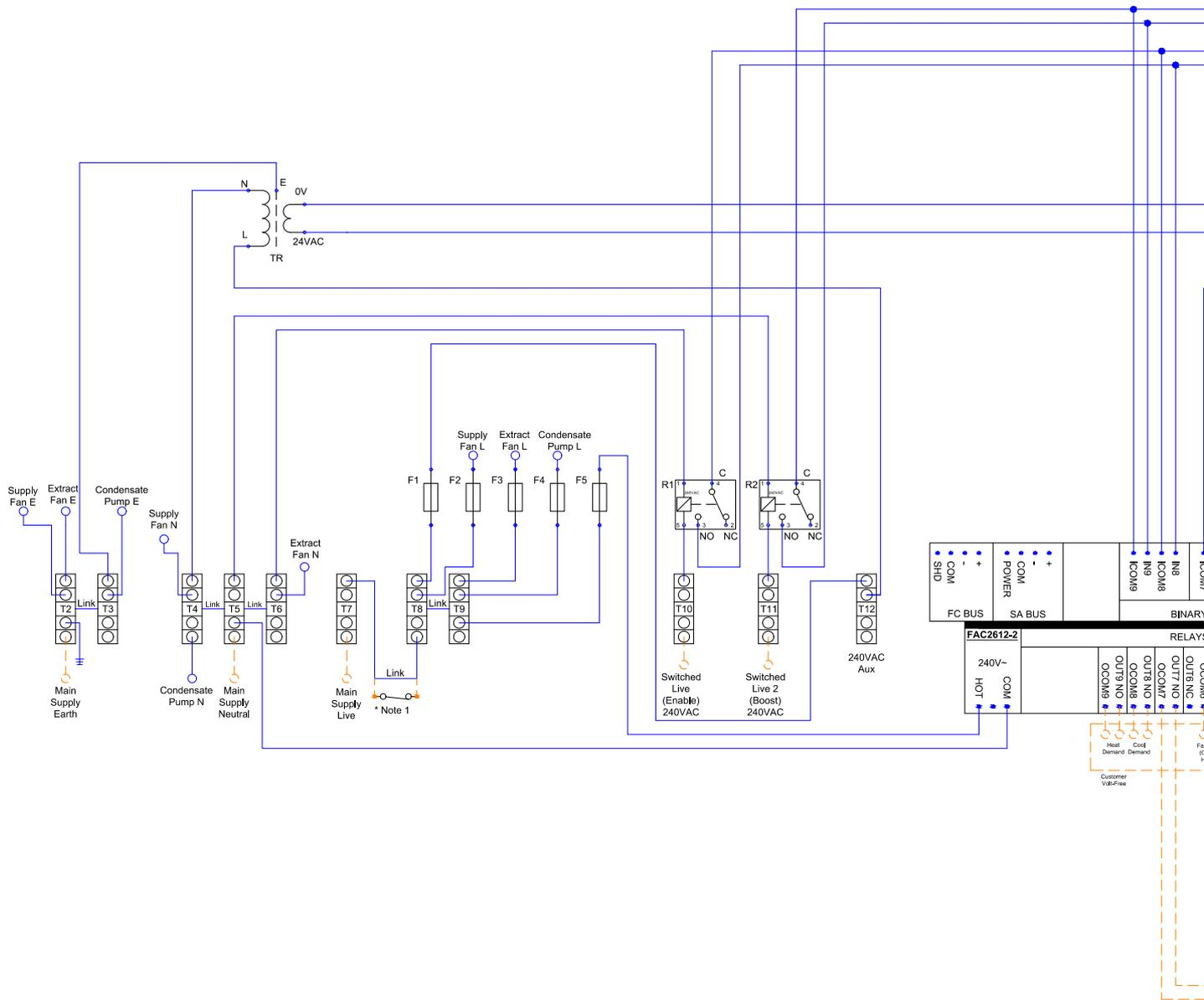
\* Note1 Emergency shutdown circuit, Break to remove power, Remove link T7-T8 to use,
