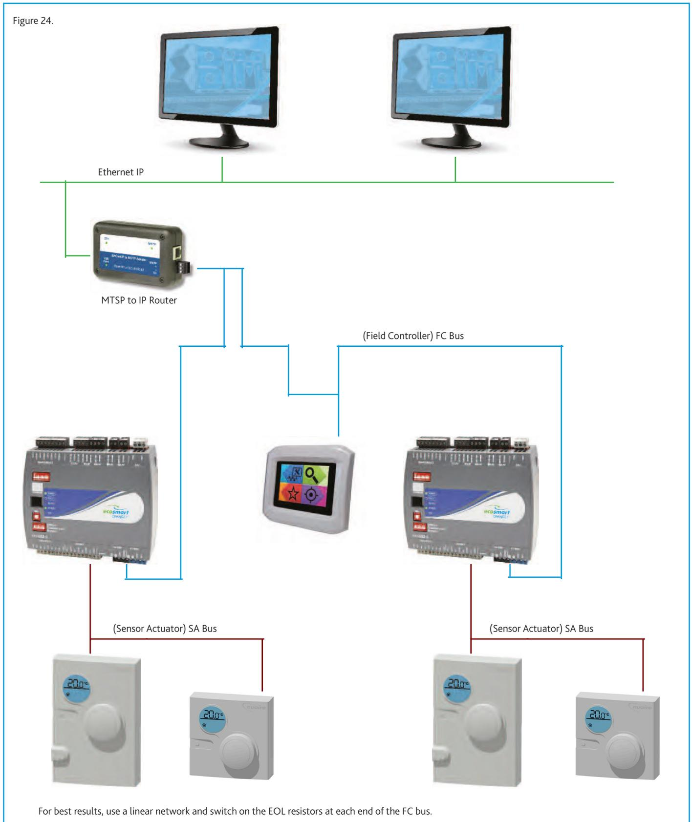
For best results, use a linear network and switch on the EOL resistors at each end of the FC bus.
