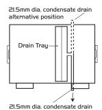
Figure 3c. Condensate pipe connection to unit and a typical example of a "U" trap drainpipe.
