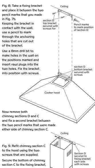
to the hood using the two screws that are supplied.
