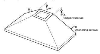
Fully tighten the support screws (A) and then screw the anchoring screws (B) through the relevant holes in the cooker hood into the wall and fully tighten.
