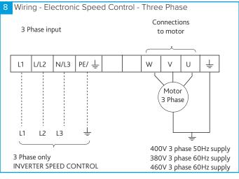
Ensure that the impeller rotation follows the label arrow indicator on the casing. Should the direction be incorrect on three phase units, reverse any two of the supply leads. Care should be taken to set correct rotation as incorrect rotation may result in damage to the motor.
