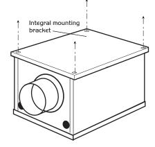
Please note that a clear space of at least 470 x 320mm is required to allow the cover to be removed and provide sufficient access for maintenance.
