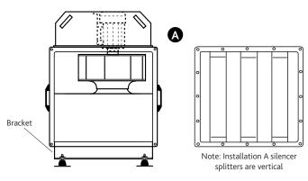
Figure 3. End view of non-recommended horizontally mounted unit installation (bracket by others).
